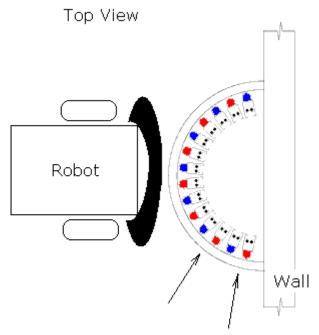
Push the disc switch from any angle
